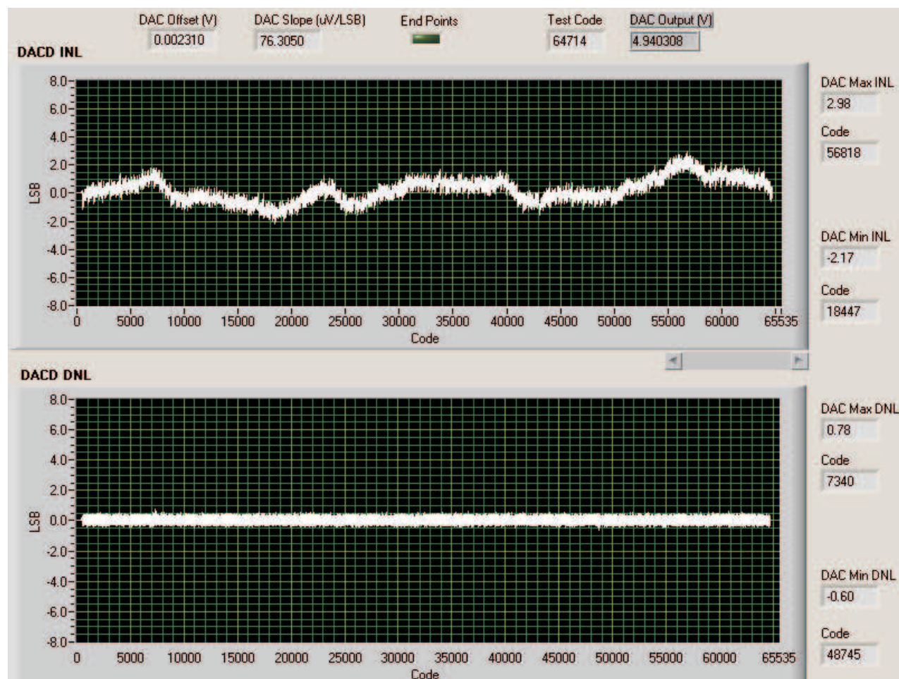
Figure 12. INL and DNL Characterization Graph of DAC D
